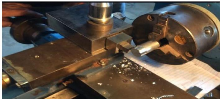
Figure1. Turning Operation at CNC Lathe (Source: KSRMCE MT LAB)
