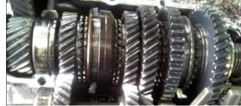
Fig.7: Gears before removing teeth.
