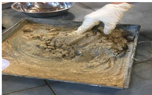
Fig. 5: Hand mixing of soil with vege-grout
