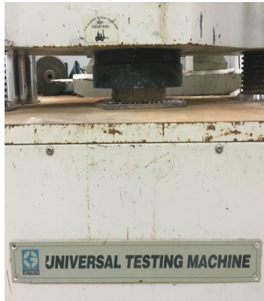
Fig. 12: Compressive strength of BVG brick for 28 days of curing.
