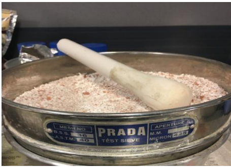
Fig. 4: Grinded eggshell filtered using sieving passing through 425 \mu m pan
