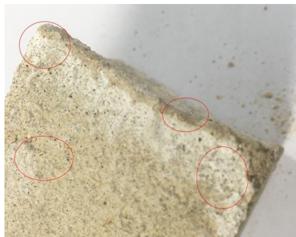
Fig. 11: Evidence of biocementation occur
