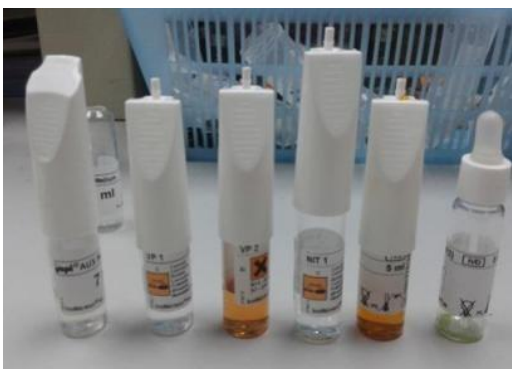
Fig. 8: API Kit 20NE(-ve) / 20E (+ve) with reagents
