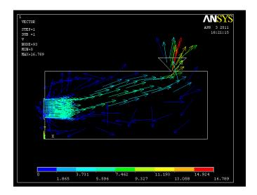
**Figure: 9** Magnitude component of flow in the hollow section of the blade.
