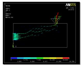
Figure: 8 Vector Component of Air Flow
