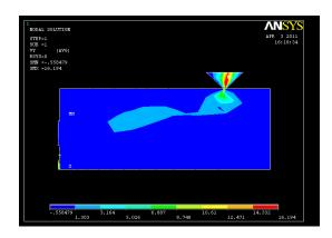
**Figure: 11** Flow of atmospheric air inside blade in Y direction
