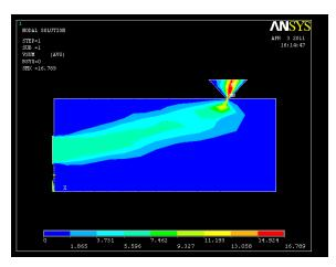
**Figure: 12** Acceleration of air at outlet with atmospheric air inlet.
