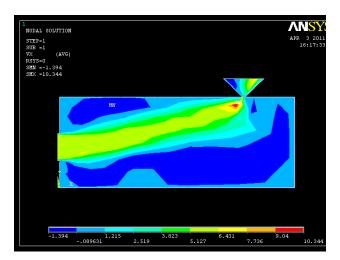
**Figure: 10** Flow of atmospheric air inside blade in X direction
