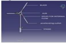
**Figure: 6** Model of Accelerated Wind Turbine
