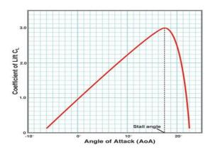
**Figure: 3**Co-efficient of lift Vs Angle of attack –graph
