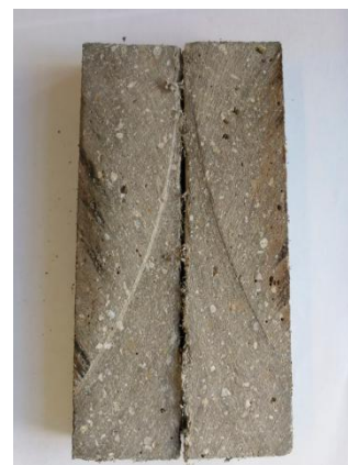
Figure 7. 3PB section samples for self-healing preparation: (a) T1; (b) T2.
