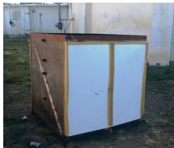
Fig.2b Constructed solar pond prototype
