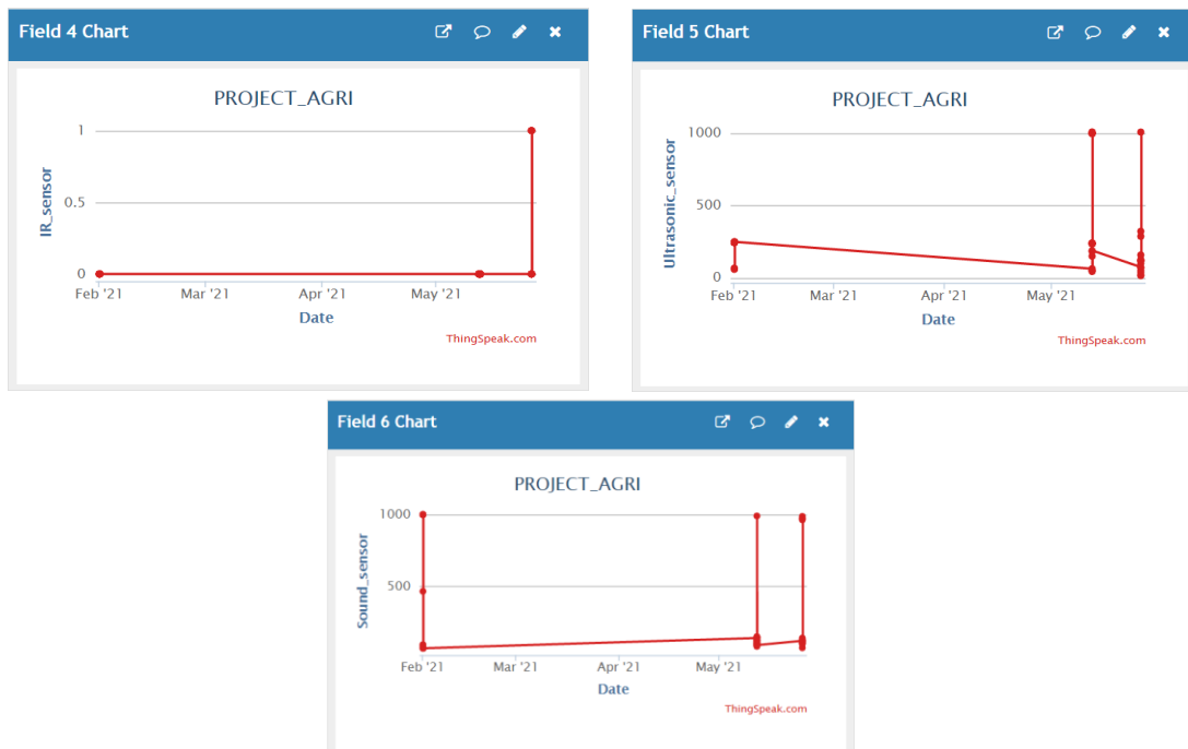
Fig 3: Output from IR, Ultra Sonic and Sound Sensor.
