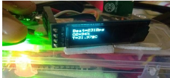
Figure7: Body temperature and blood oxygen level monitoring device output
