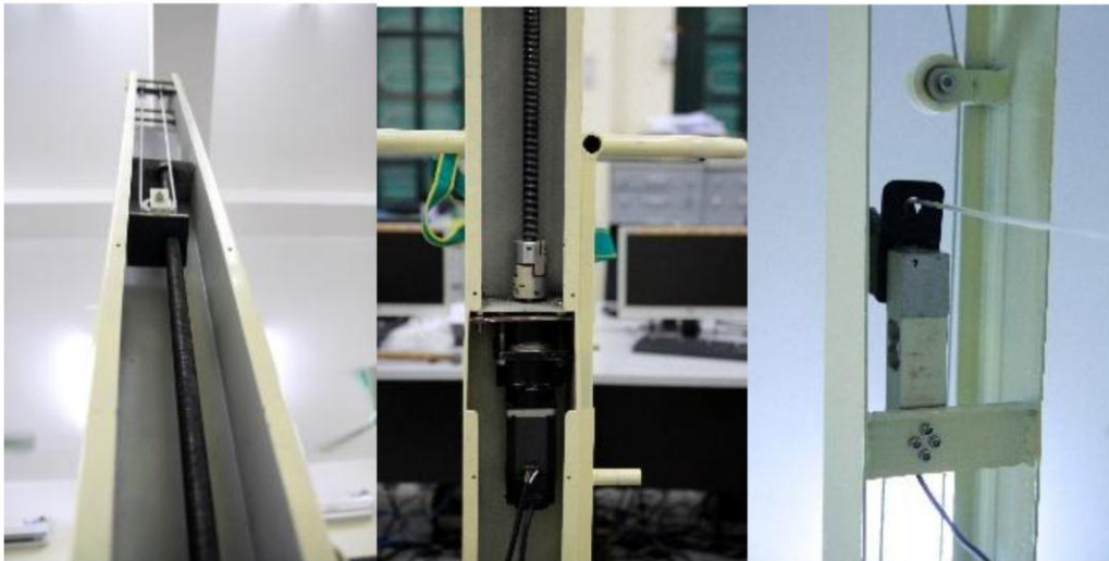
Figure 9: Mechanical mechanism for generating and measuring the driving force
