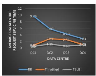
Figure. 8 Results showing the average data centre request servicing time of load balancing algorithms such as RR, Throttled and proposed TBLB.
