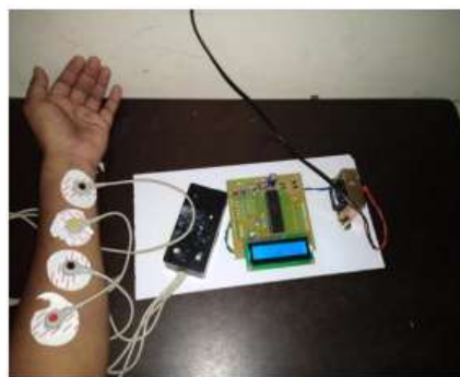
Fig. 2. Impedance Plethysmography -Hardware Implementation Circuit
