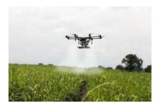
Fig. 6. Crop spraying using drone
