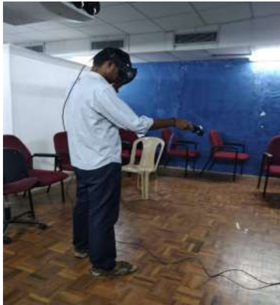
Figure 3. User interacting with the help of HTC-Vive and accessories for teleportation The user can directly switch to the next room for navigation just by pressing the appropriate button in the accessories of HTC-Vive.
