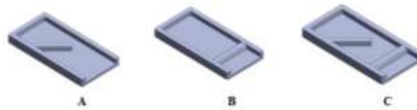
Fig 6. Different hopper models. A: Model 1 – Wiper blade B: Model 2 – Barrier. C: Combination of Model 1 and Model 2 – Wiper blade and barrier.
