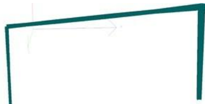
Figure 5: Tapering of rafters of the Pre-Engineered Building
