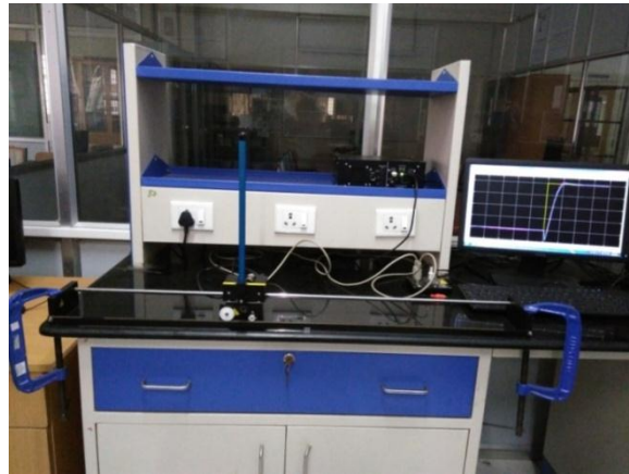
Fig. 3. Single Inverted Pendulum hardware set-up
