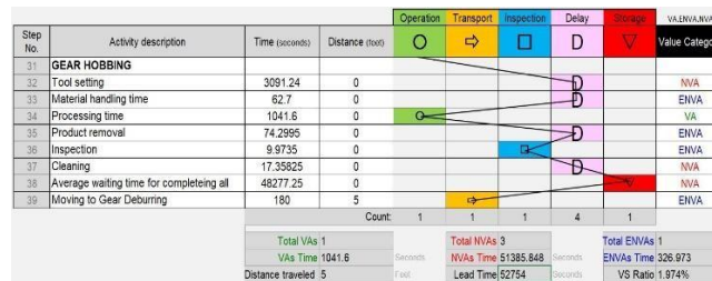
Fig.9. Process flow chart for Gear hobbing of gear shaft
