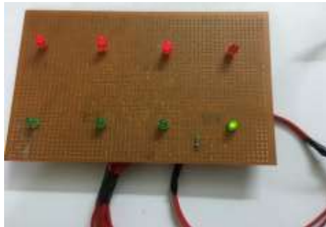
Figure 9: Signal On North Side Turns On (Emergency)
