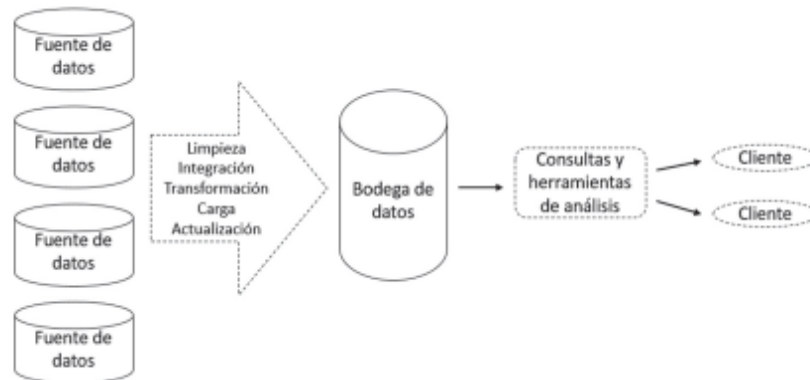
Figure 2: Flow of an ETL process associated with a datawarehouse
