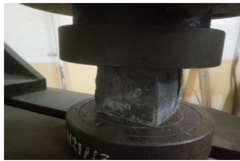
Failure of specimen
