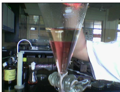
Figure 2: Extraction of Prodigiosin
