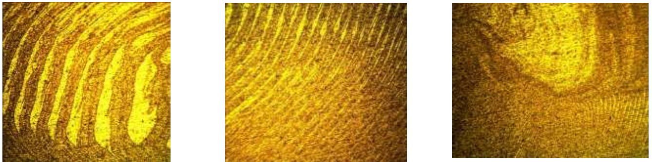
(a) INTERFERE ZONE 5083-O (b) INTERFERE ZONE 6061-T6 (c) WELD REGION
