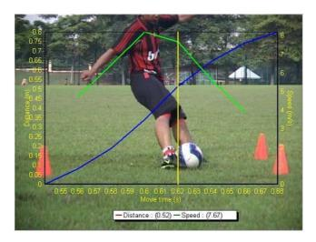
Figure 4: Velocity Versus Time
