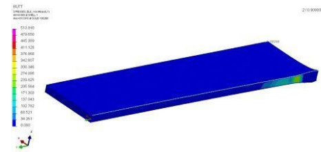
Figure 7 Contour plot of residual stress distribution at 64 A
