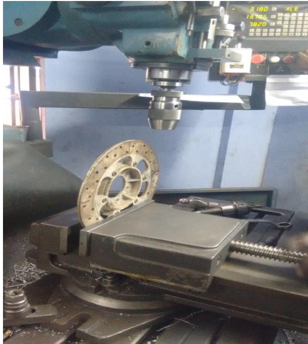
Figure 3 Drilling of Holes in Disc Brake
