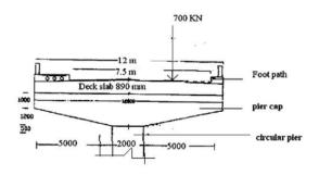
Considering one meter width of cantilever slab the dead load moment at the fixed end of the
