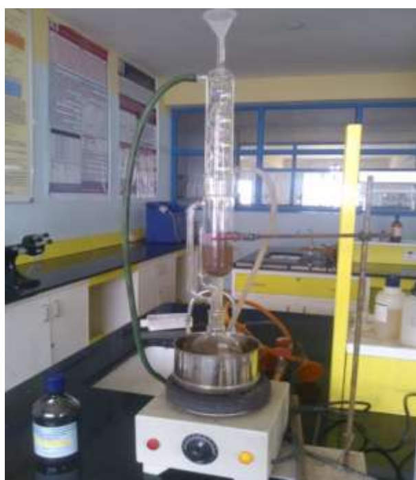
Figure: 1 Soxhlet apparatus used for extraction of crude drug from Coriandrum Sativum seeds Column chromatography for isolation
