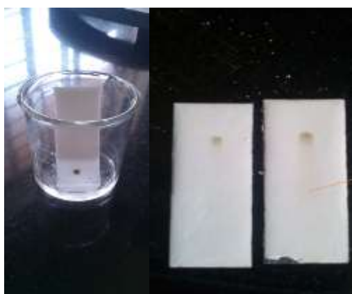
Figure: 6 Development of TLC plate and Detection of TLC plate by vanillin which shows the presence of linalool
