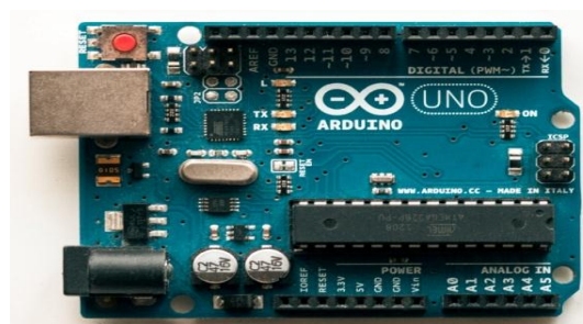
Figure 2. Arduino Uno Microcontroller based ATmega328
