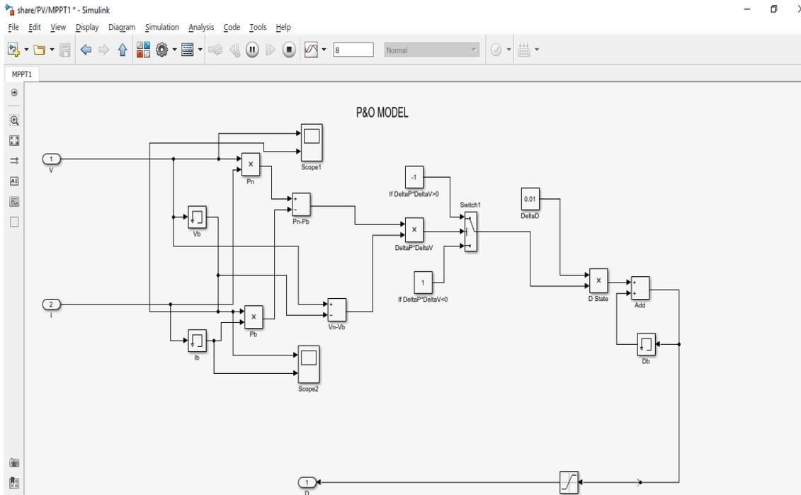
Fig 5. MPPT Simulation Diagram
