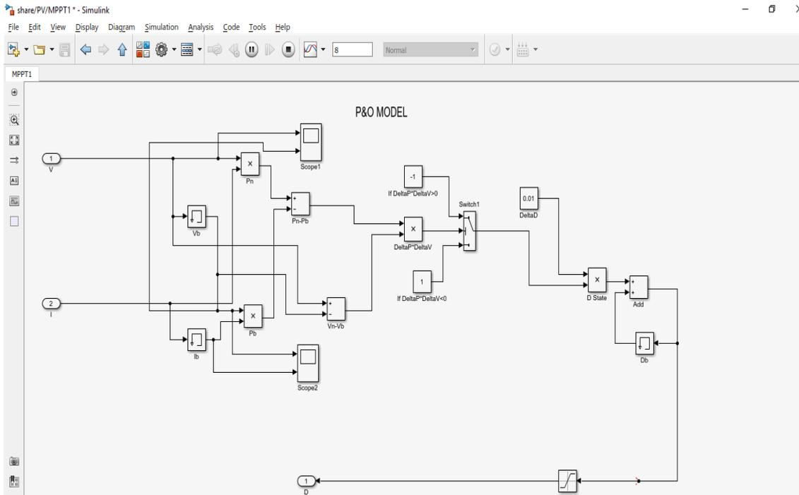
Fig 5. MPPT Simulation Diagram
