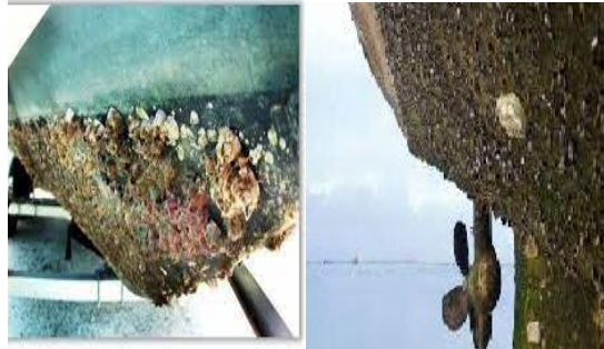
Fig No.1 Images showing presence of biofouling in the ship hull
