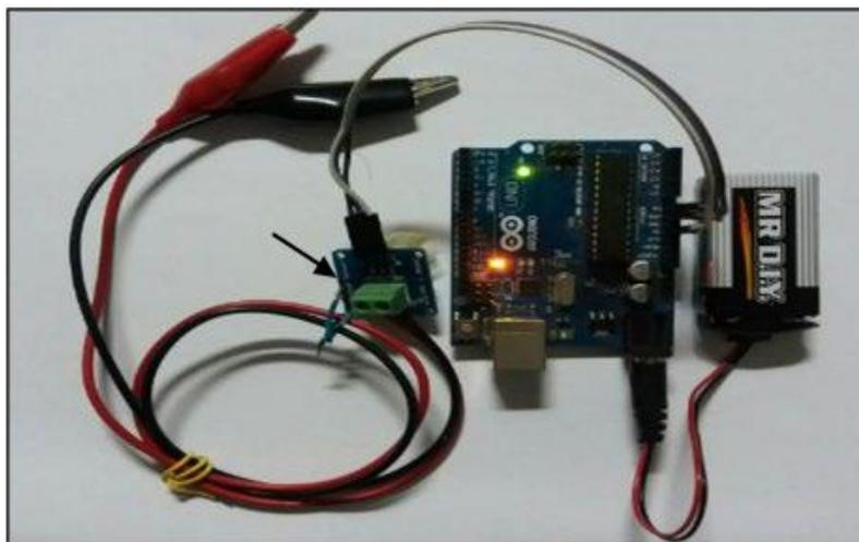
Figure 2: Battery voltage measurement using voltage sensor Circuit.
