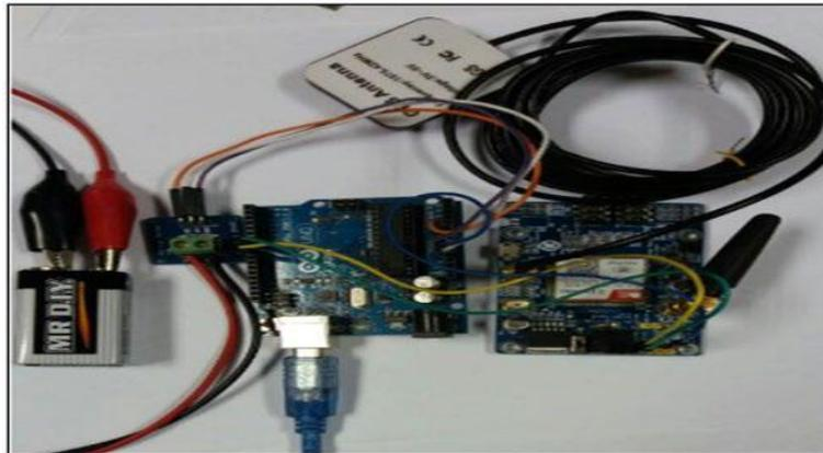
Figure 3: Hardware for the developed battery monitoring system consists of voltage sensor and SIM808 GSM/GPRS/GPS module
