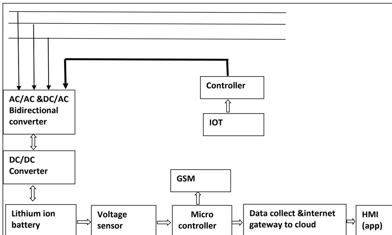
Figure 1: Block diagram of overall proposed design
