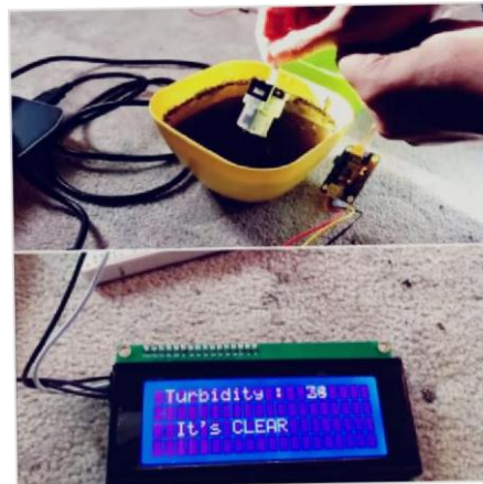
FIGURE 3: Turbidity sensor for the detection of the turbidity.
