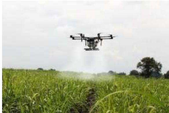
Fig. 6. Crop spraying using drone
