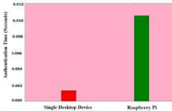
Fig.9.Comparison For Authentication Time Based On H/W Implementation
