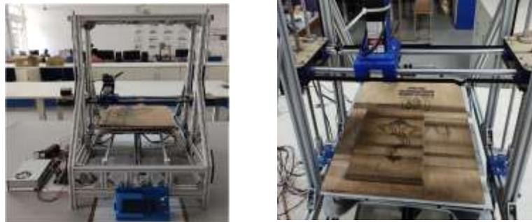
Fig. 2. Laser Engraving Setup Modules For Multipurpose Cnc Machine.
