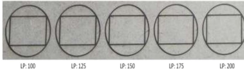
Fig. 3a. Output For Various Laser Power For The Travel Speed: 3000 Mm/Min; Pass: 1 And Pass Depth 1 Mm.
