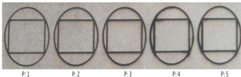
Fig. 3c. Output For Various Passes For The Laser Power: 100 W; Travel Speed: 3000 Mm/Min And Pass Depth 1 Mm.
