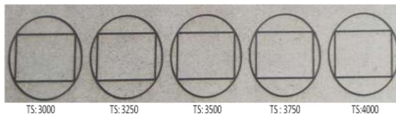
Fig. 3b. Output For Various Travel Speed For The Laser Power: 100 W; Pass: 1 And Pass Depth 1 Mm.
