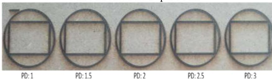
Fig. 3d. Output For Various Pass Depth For The Laser Power: 100 W; Travel Speed: 3000 Mm/Min And 2 Passes.
