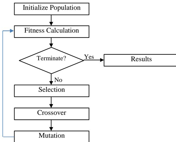
Fig 3 Flow diagram of genetic algorithm
