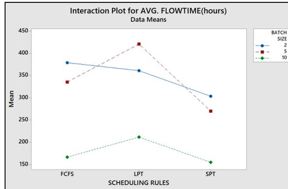
Fig. 15 Interaction Plot for Average flow time
