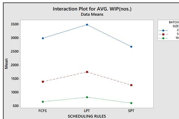
Fig. 13 Interaction Plot for Average WIP
