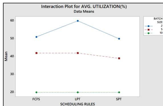
Fig. 14 Interaction Plot for Average utilization
