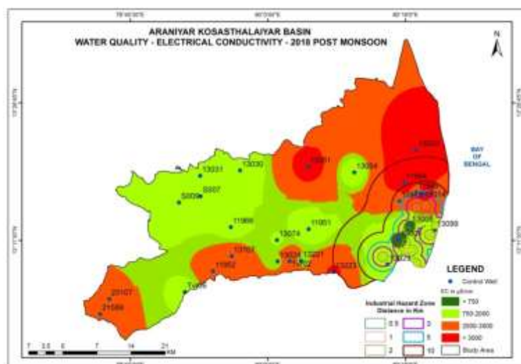
Fig.5B E.C with Industrial Hazard Zone - Post Monsoon
