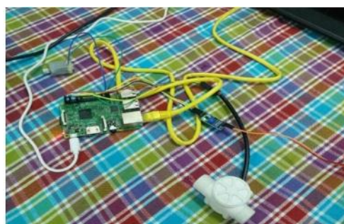
Figure 2.3: Moisture Sensor, motor, water pump interfaced to raspberry pi
