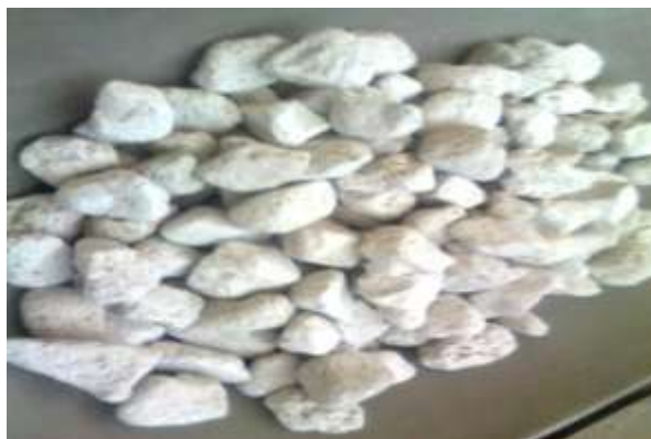
Fig: 3.1 Light weight Aggregate (Pumice) Table 3.4: Sieve Analysis of (Pumice) Aggregate
