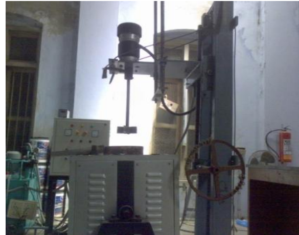
Fig. 1 Stir casting process set-up
