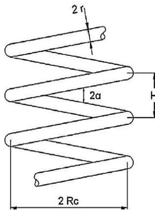
**Figure : 1** Geometry of helical tube
