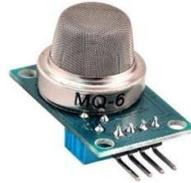
The concentration range of MQ-6 gas sensor is 200-1000 ppm. The sensor has fast response time and high reliability and efficiency range up to 90% especially of LPG gases [4]. The power need by the sensor is 5V.
