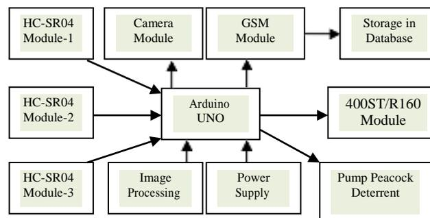
**Fig. 4.** Architecture of Crop Protection from Peacock
