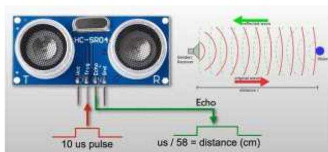
**Fig. 3.** Ultrasonic Sensor for detecting animals
