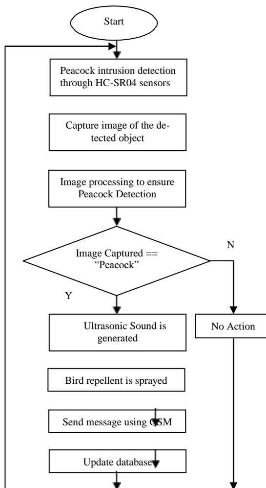
**Fig. 5.** Flow Diagram depicting Crop Protection against Peacock
