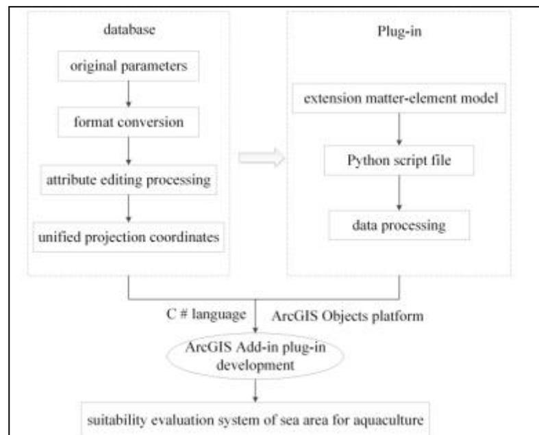
Fig.1 System design flow chart
