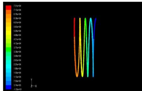
**Figure: 7** Contour of pressure for hot fluid
