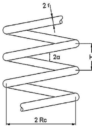
**Figure : 1** Geometry of helical tube
