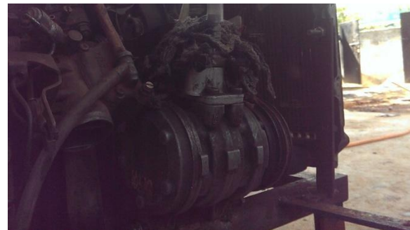
Figure-3. The electromagnetic clutch type compressor
