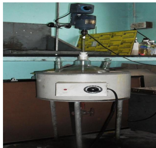
Fig3.1 Photographic view of transesterification set up
